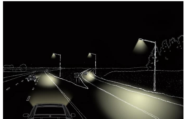
Figure 7: Partial Interchange Lighted Off-Ramp, Isometric View
